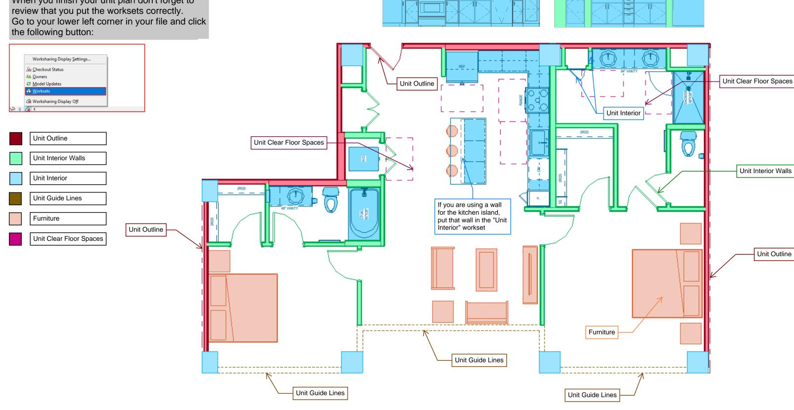
Walls and ceiling that you are using for the kitchen dropped ceiling you shall use the "Unit Interior" workset
